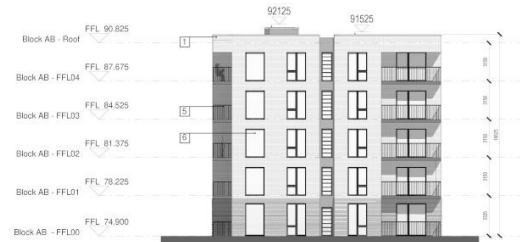
4 Proposed North Elevation - Block AB 1 : 200
