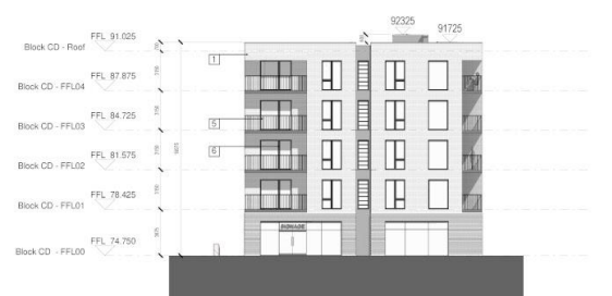
4 Proposed North Elevation - Block CD 1 : 200
