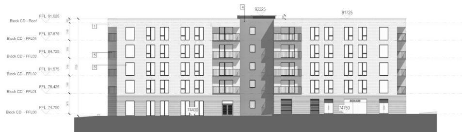
5 Proposed East Elevation - Block CD 1 : 200
