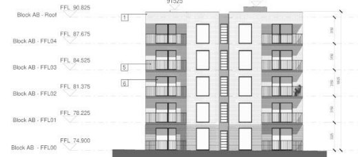
2 Proposed South Elevation - Block AB 1 : 200
